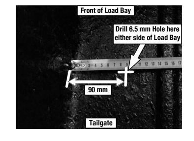
(**H**) Secure the two D-rings (Item 32 received with SSDS401) to the inside of the vehicle's load bay by bolting through the two 6.5 mm holes drilled in Step 2G, using two M6 x 25 Hex Bolts, four M6 x 19 Flat Washers and a two M6 Nyloc Nuts (Items 33, 34, 35 received with SSDS401) as shown.
