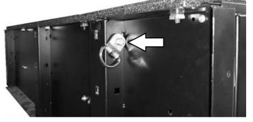
(H) Working at the front of the load bay, make a mark on either side of the load bay, 160 mm in from the rear of the load bay and 90 mm in from the side of the load bay. Drill a 6.5 mm hole on each of your markings
