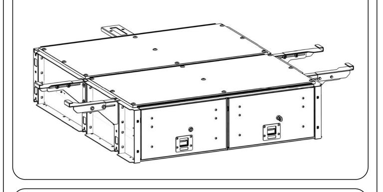
(**C**) Position the Corner Wing Assemblies from Step 2B over the corners of the Drawer as shown. Secure the Assemblies to the Drawer using the remaining M6 x 20 Hex Bolts, M6 x 19 Flat Washers and M6 Spring Washers. When securing the TOP mounting on the side of the Drawer, loosely fasten a D-Ring (Item 4) to each corner as shown.
