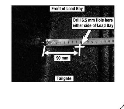
(**I**) Secure the two D-rings (Item 32 received with SSDS401) to the inside of the vehicle's load bay. You will be bolting through the two 6.5 mm holes drilled in Step 2G using a two M6 x 25 Hex Bolts, four M6 x 19 Flat Washers and a two M6 Nyloc Nuts (Items 33, 34, 35 received with SSDS401) as shown.
