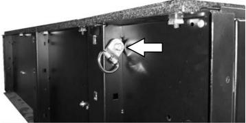
( H ) Working inside the loadbay, just below the wheel arches towards the rear of the vehicle, measure and mark the load bay either side as indicated below. Drill a 6.5mm hole on each of your markings.
