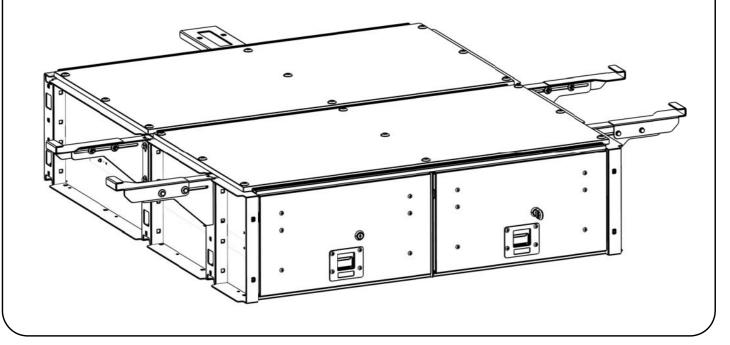
Position the Corner Wing Assemblies from Step 2B over the corners of the Drawer as shown. Secure the Assemblies to the Drawer using the remaining M6 x 20 Hex Bolts, M6 x 19 Flat Washers and M6 Spring Washers. When securing the TOP mounting on the side of the Drawer, loosely fasten a D-Ring (Item 4) to each corner as shown.
