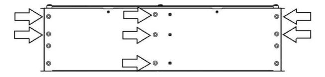
(F) Using six M6 x 20 Hex Hex Bolts, six M6 Spring Washers and six M6 x 19 Flat Washers removed in Step 2E, secure the Rear Support (Item 23) to the back of the Drawer System as shown.
