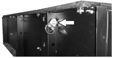
( H ) Working at the front of the load bay, make a mark on either side of the load bay, 160 mm in from the rear of the load bay and 90 mm in from the side of the load bay. Drill a 6.5 mm hole on each of your markings
