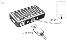
Turn on the USB charging by pressing the USB Power ON/OFF Button on the powerstation go rugged compact.
